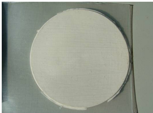
Fig. 1. Appearance of a PMMA membrane prepared with the CO 2 -assisted phase inversion method.
